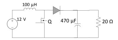
Q.50 The PEAK-TO-PEAK source current ripple in Amps is
